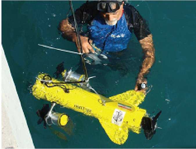
Fig. 4. The proposed ROV and incorporated diagnostic arm for inspection and NDT of a quay wall in Shahid-Rajaei harbor
