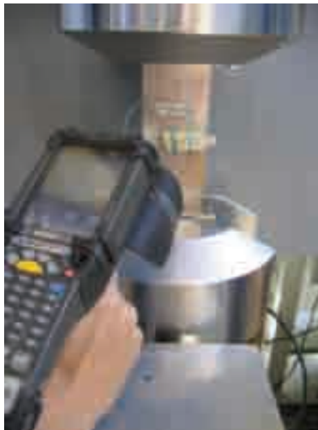
Fig. 20. Illustration of an RFID-based crack detection approach.
